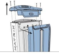
Do not fully tighten frame connectors until assembly is complete. Vibra-Tite 135 Red Gel or equivalent must be used on all fasteners that are not assembled with Nyloc Nuts.
