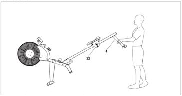
To move the machine, lift the rear support tube until the moving wheel on the front support tube touches
